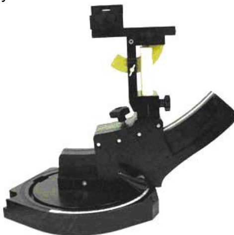
Device holder supplied by SPEAG
