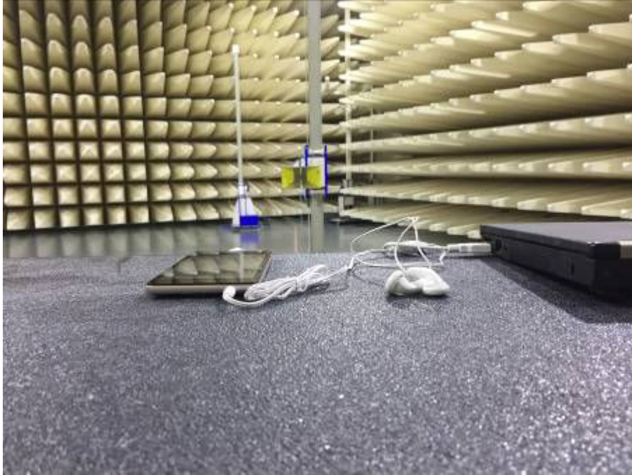
Pic6: Radiated Emissions Test Setup (with laptop)
