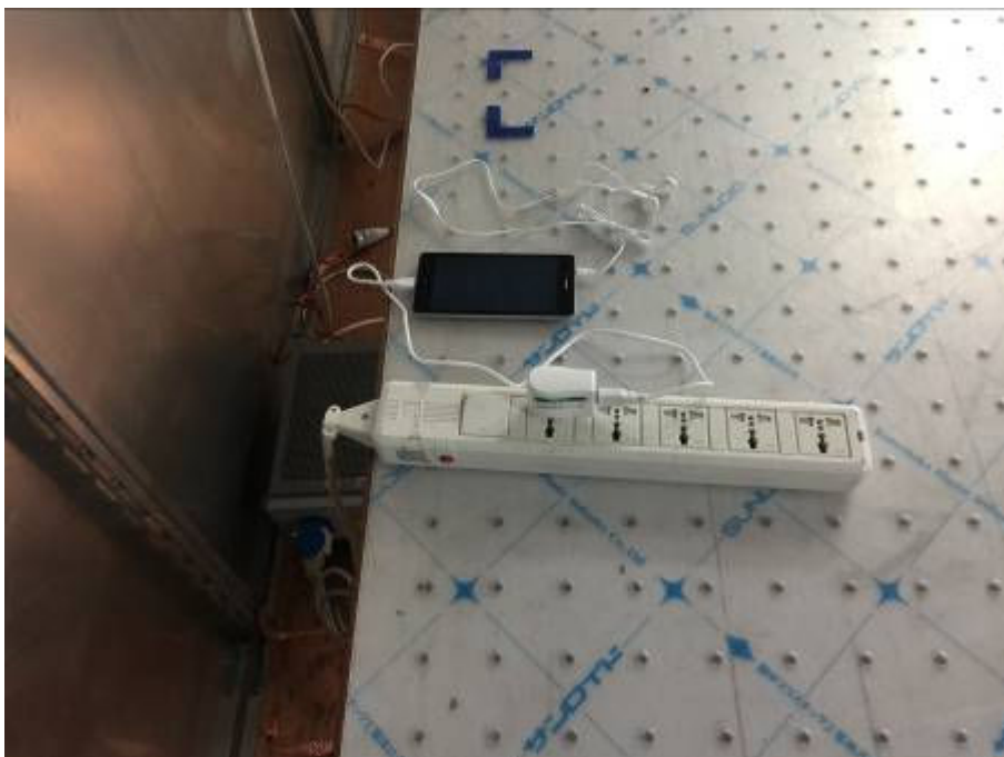
Pic9: Conducted Emissions Test Setup (with charger)
