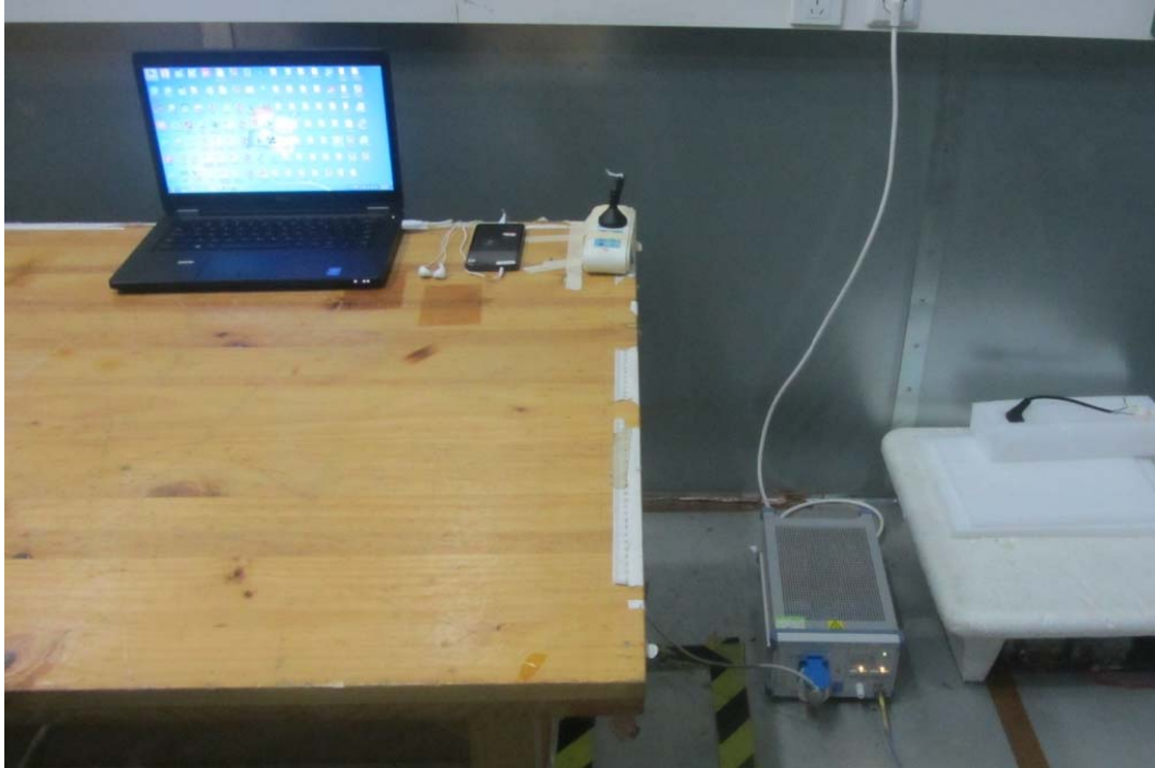
Picture 2 Conducted Emission Test Setup
