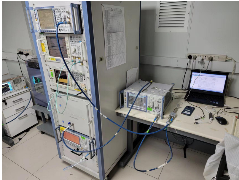
RF Conducted Test setup (GSM/WCDMA/LTE)
