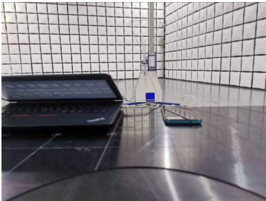
Radiated Emissions Test Setup (with laptop) (30-1000MHz)
