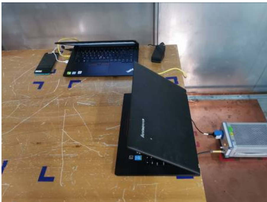
Conducted Emissions Test Setup (with laptop)
