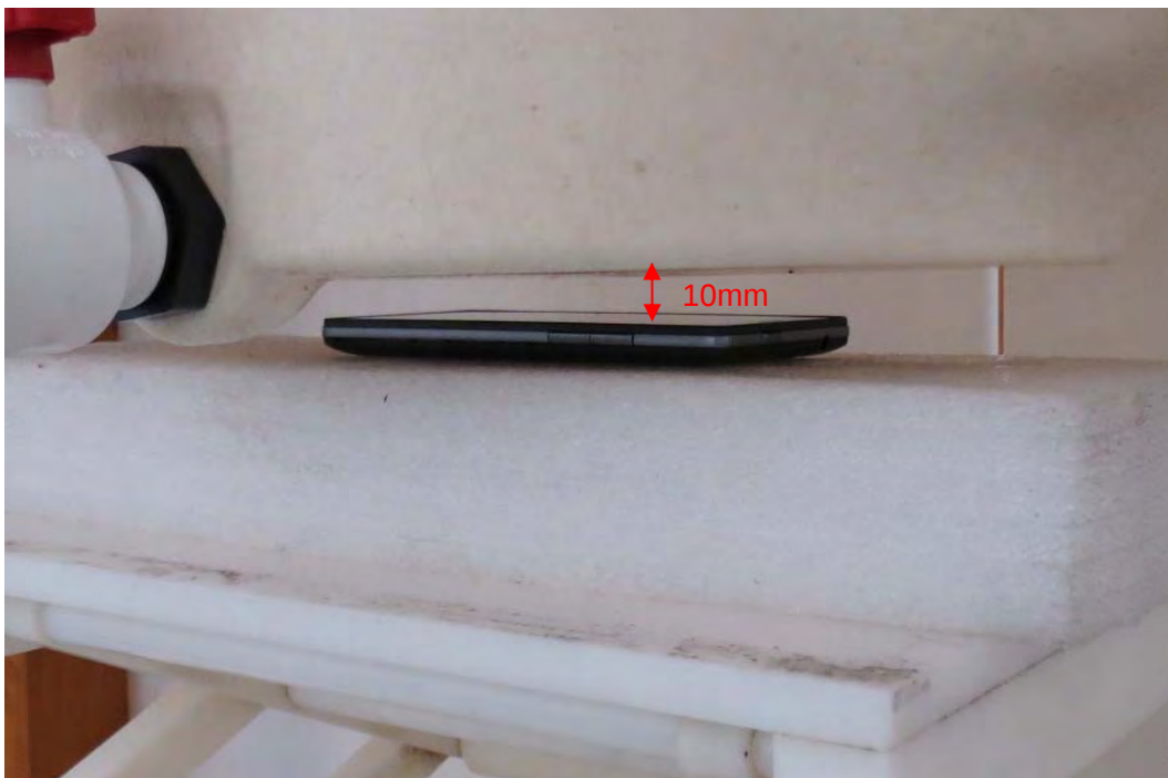
Picture 19: Front Side, the distance from handset to the bottom of the Phantom is 10mm Z815 (RXC1512-0230SAR01R1)
