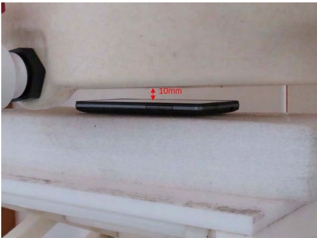
Picture 27: Front Side, the distance from handset to the bottom of the Phantom is 10mm Z815 (RXA1611-0257SAR01R2)/ Z815 (RXA1707-0217SAR)
