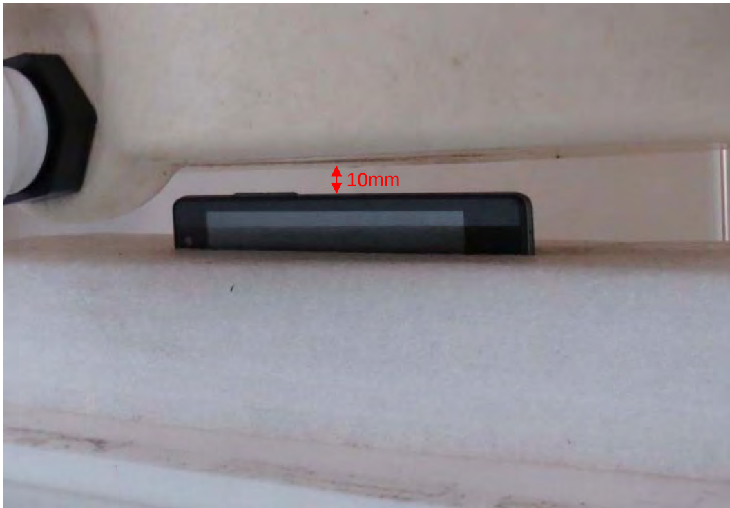
Picture 28: Right Side, the distance from handset to the bottom of the Phantom is 10mm Z815 (RXA1611-0257SAR01R2)/ Z815 (RXA1707-0217SAR)
