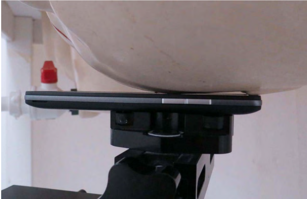
Picture 24: Left Hand Touch Cheek Position Z815 (RXA1611-0257SAR01R2)/ Z815 (RXA1707-0217SAR)
