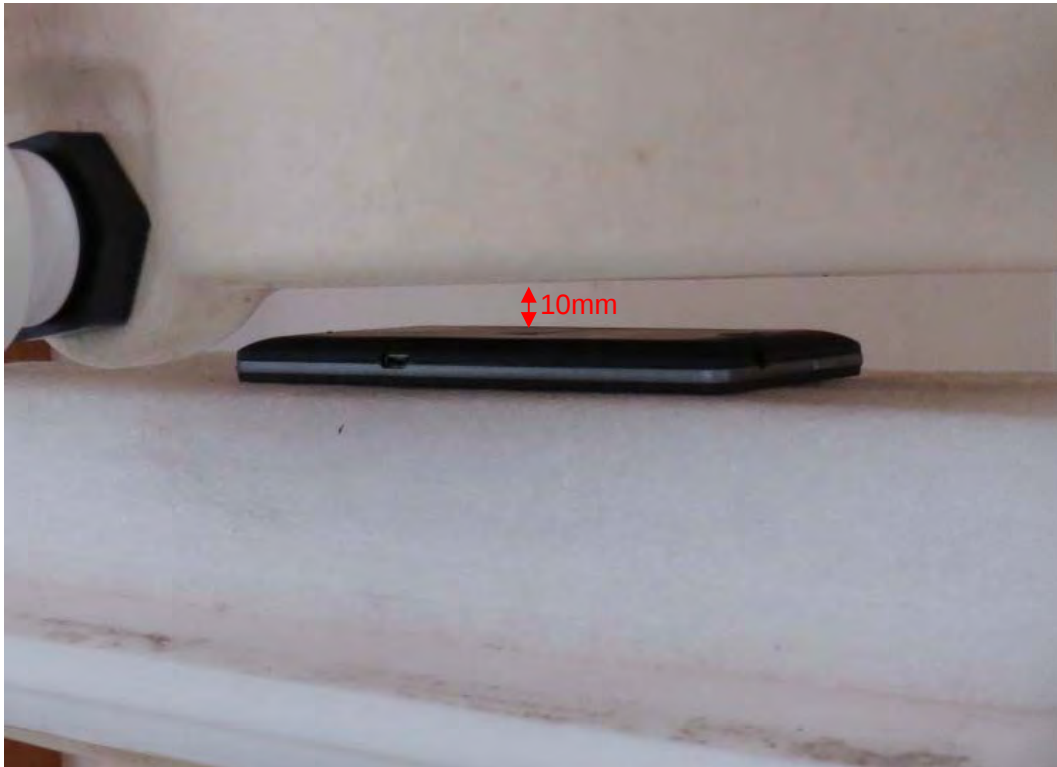
Picture 26: Back Side, the distance from handset to the bottom of the Phantom is 10mm Z815 (RXA1611-0257SAR01R2)/ Z815 (RXA1707-0217SAR)
