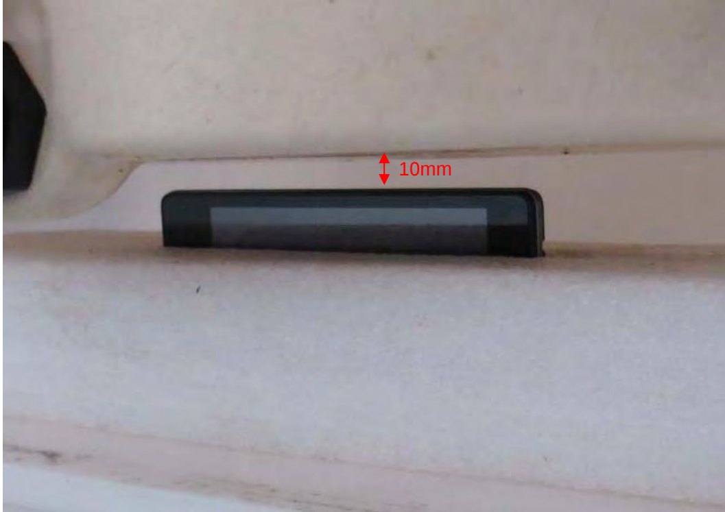
Picture 20: Left Side, the distance from handset to the bottom of the Phantom is 10mm Z815 (RXC1512-0230SAR01R1)
