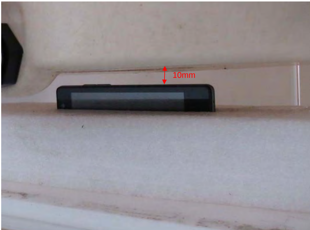
Picture 21: Right Side, the distance from handset to the bottom of the Phantom is 10mm Z815 (RXC1512-0230SAR01R1)
