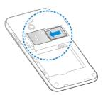
Insert the battery by aligning the metal contacts on the battery with the metal contacts in the battery compartment. Gently push down on the battery until it clicks into place.
