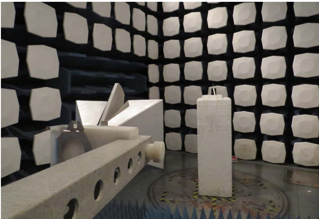
Picture 2: Radiated Spurious Emissions Test setup
