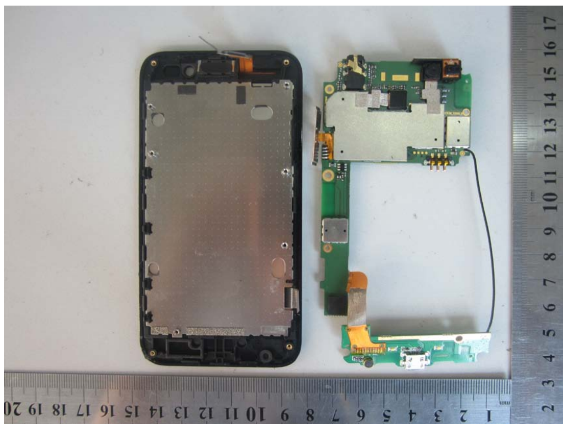
2. Mainboard front view with shielding
