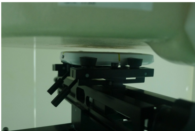
Front of the DUT with Phantom 0.5 cm Gap
