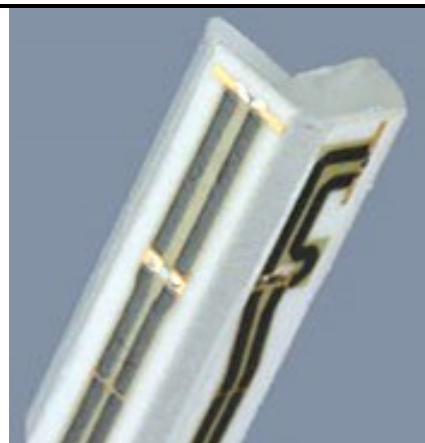
Fig 5.2 Photo of E-field Probe
