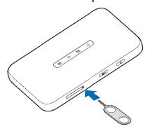
2. Remove the SIM tray. Place the nano-SIM card on the tray as shown. Carefully, slide the tray back into place.
