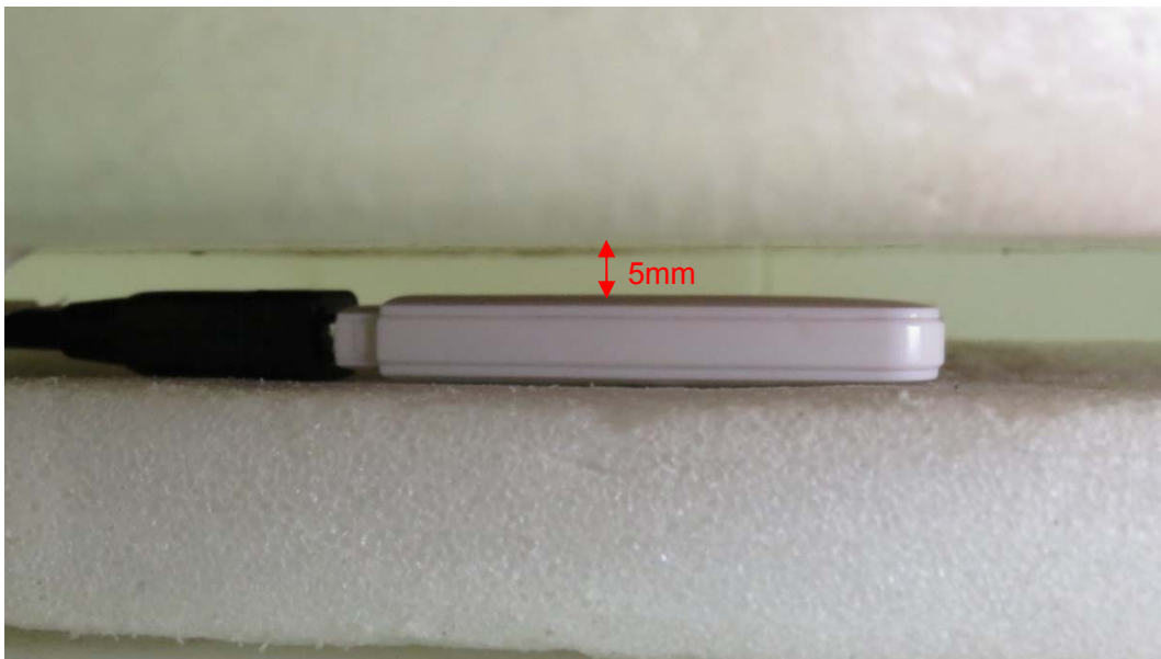
Picture 8: Front Side, the distance from EUT to the bottom of the Phantom is 5mm
