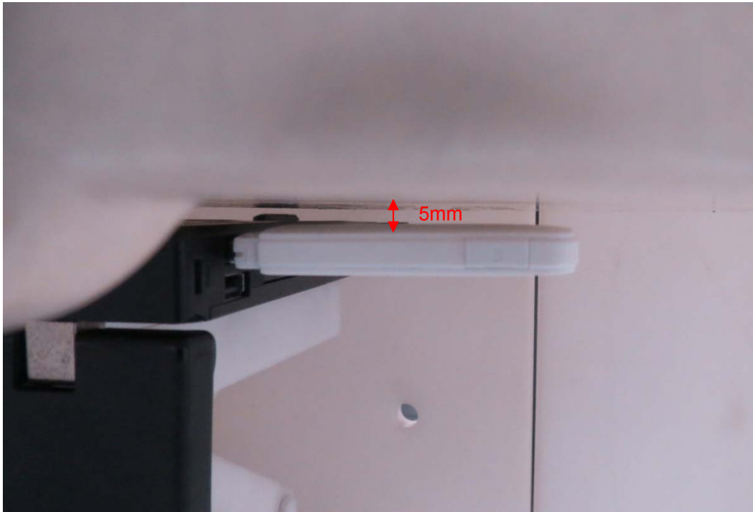
Picture 7: Back Side, the distance from EUT to the bottom of the Phantom is 5mm
