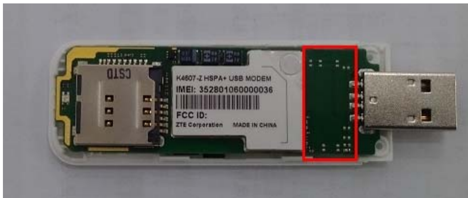
Main antenna(TX and RX)
