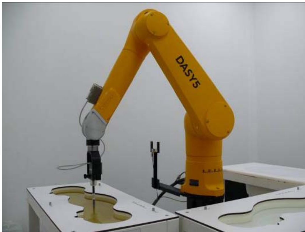
Picture 3: Specific Absorption Rate Test Layout
