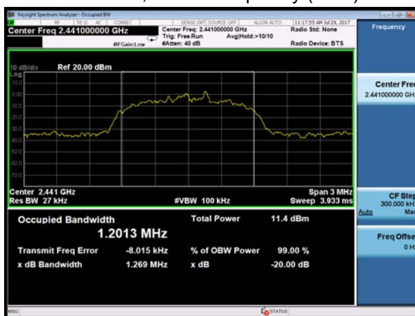
BT 2DH5 CH39, Carrier frequency (MHz): 2441
