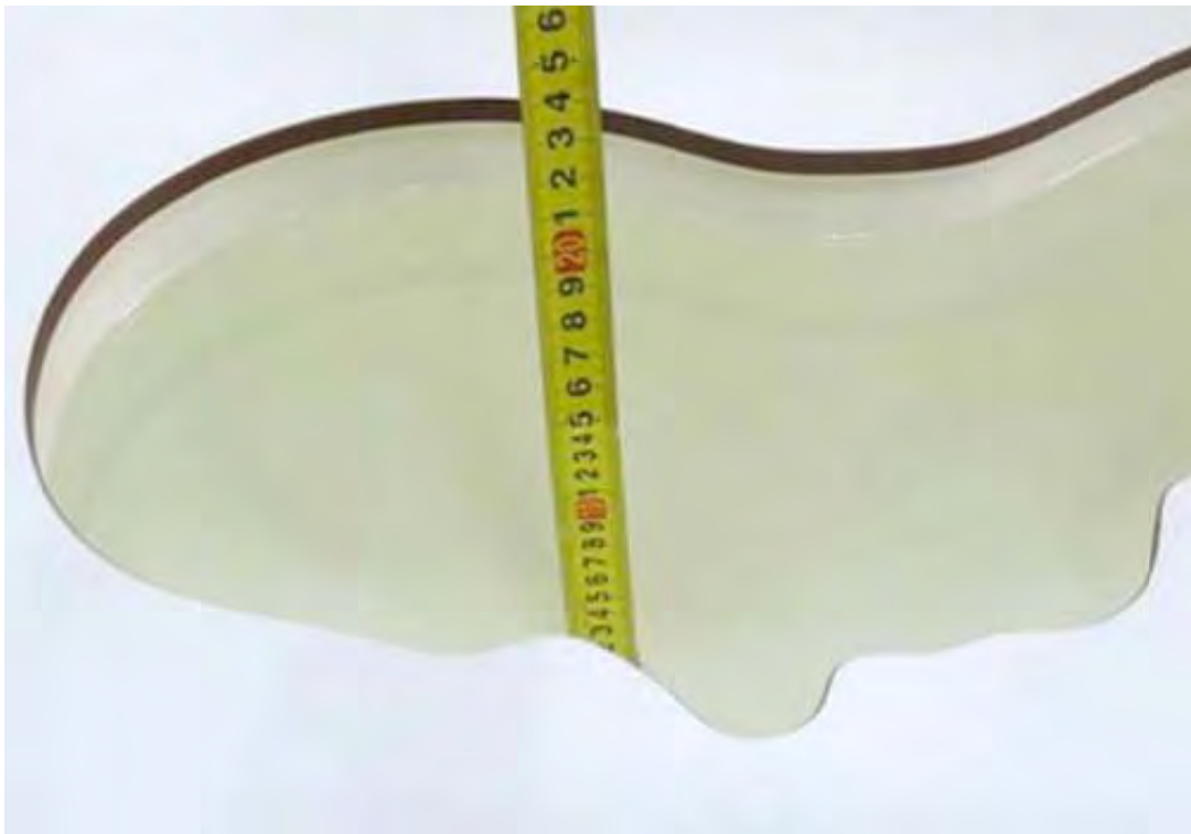
Picture 5: Liquid depth in the head Phantom (2450 MHz, 15.4cm depth)
