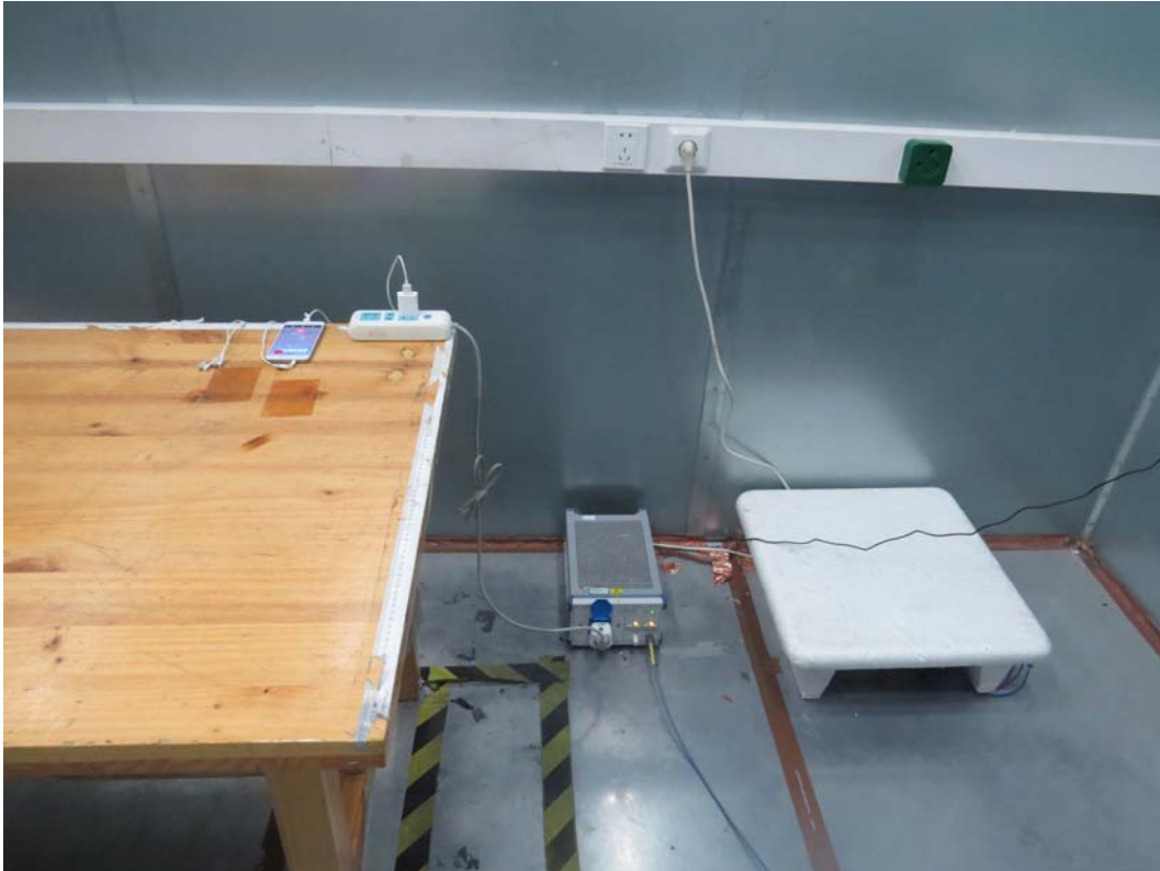
Picture 3 Conducted Emission Test Setup
