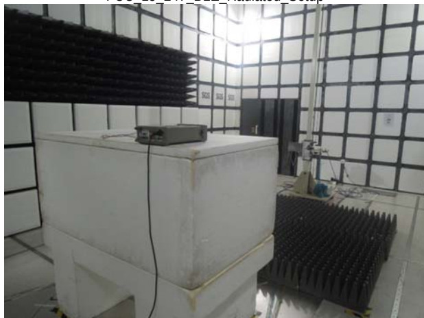
FCC 15 247 BLE Radiated Setup
