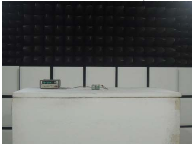
FCC 15 247 BLE Radiated Setup
