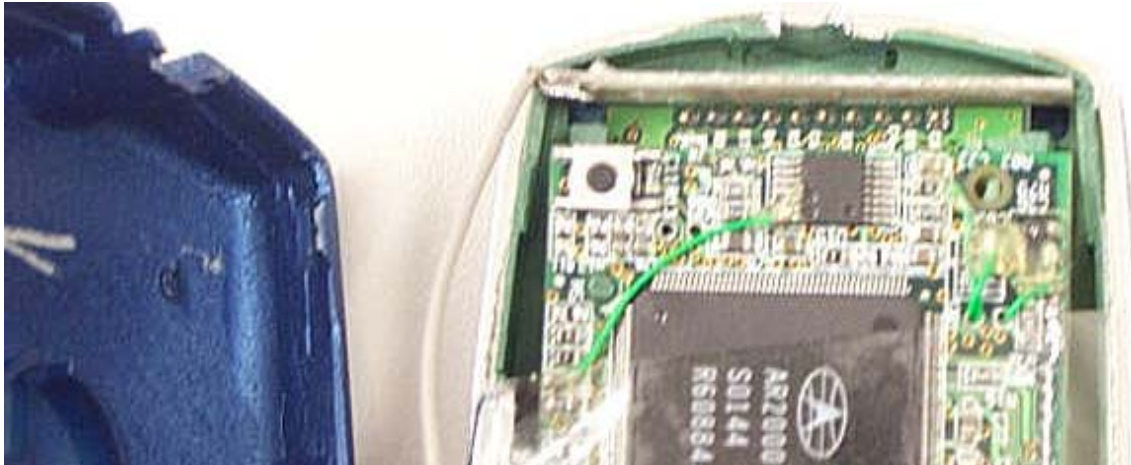
Example of Application, Antenna should be far from ground plane or metal shielding
