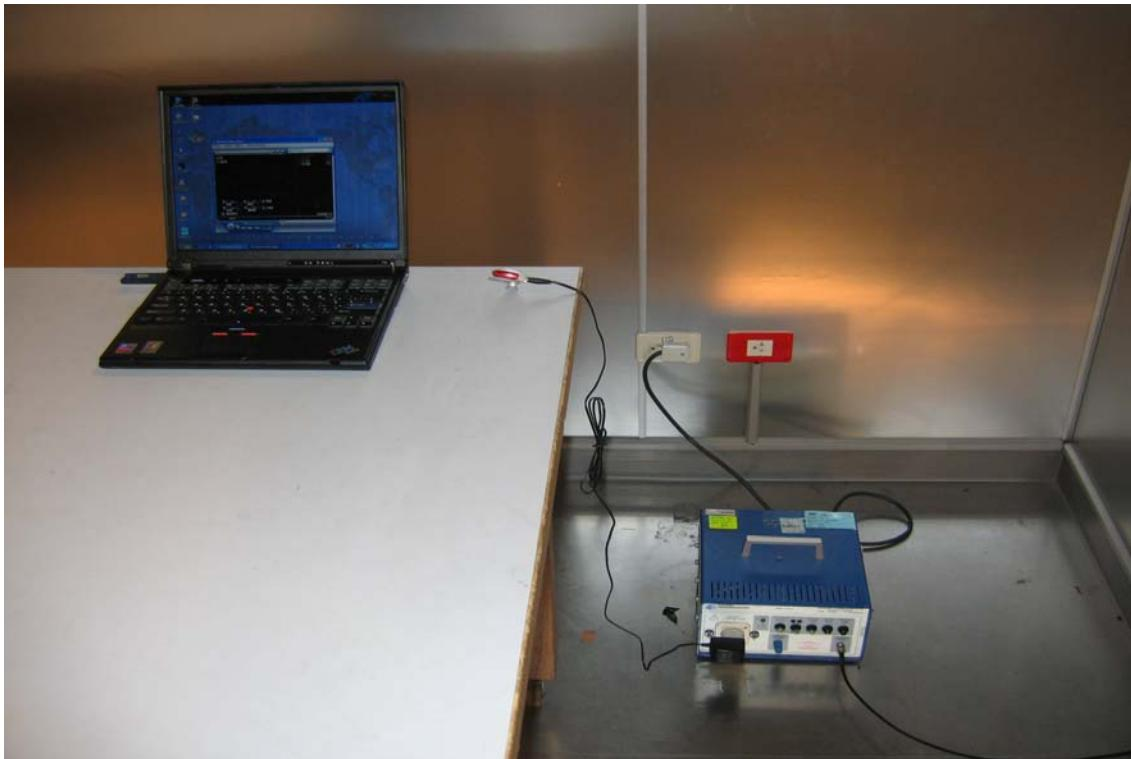
**Conducted Emission Set up Photo**
