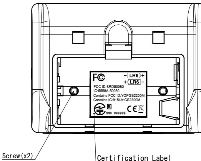
The FCC/CE certification label is attached inside the battery box.
