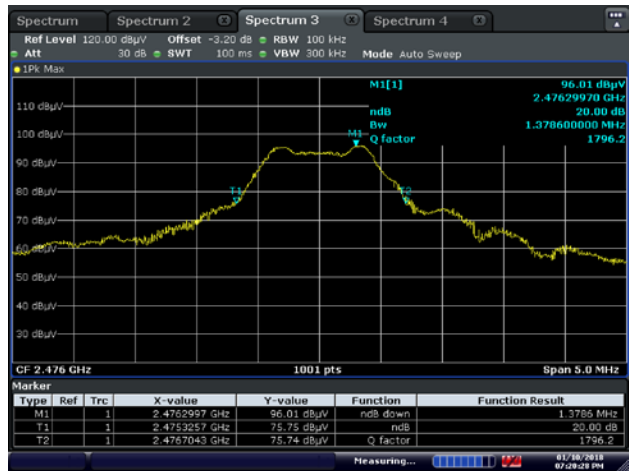
Figure 8.1-3: 20 dB Bandwidth, High CH
