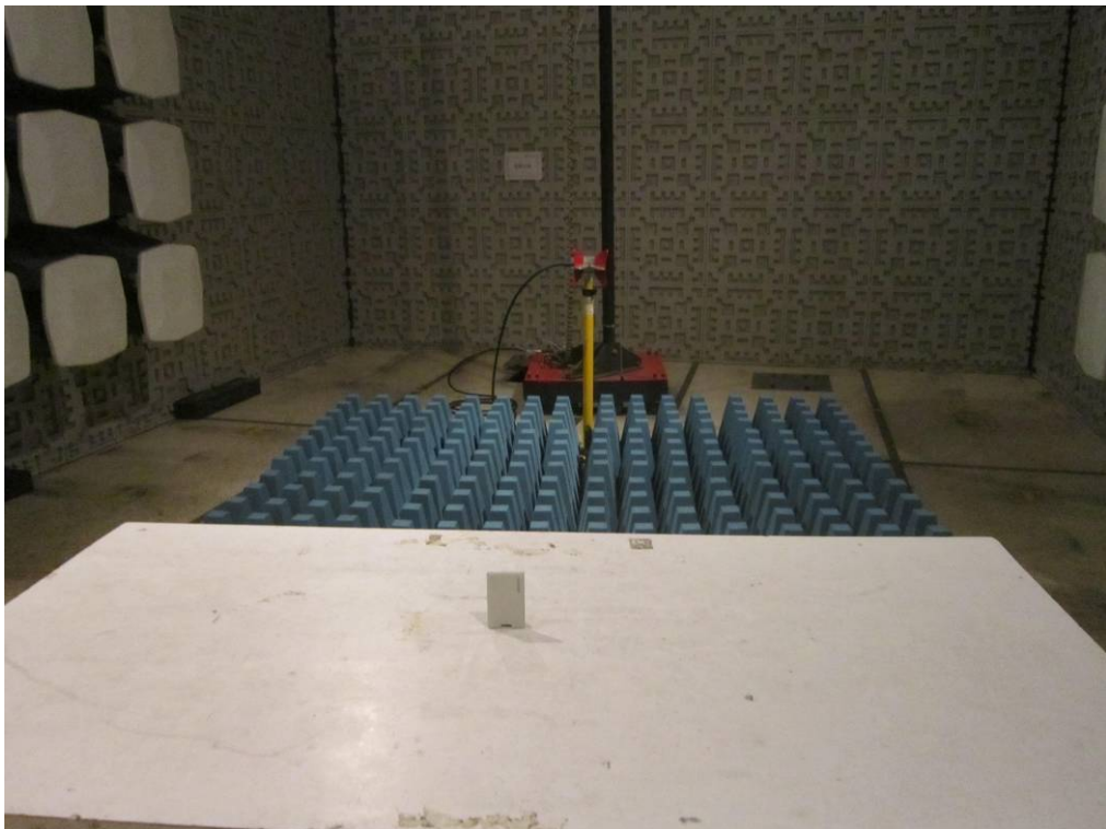
TEST SETUP OF RADIATED EMISSION (above 1GHz)
