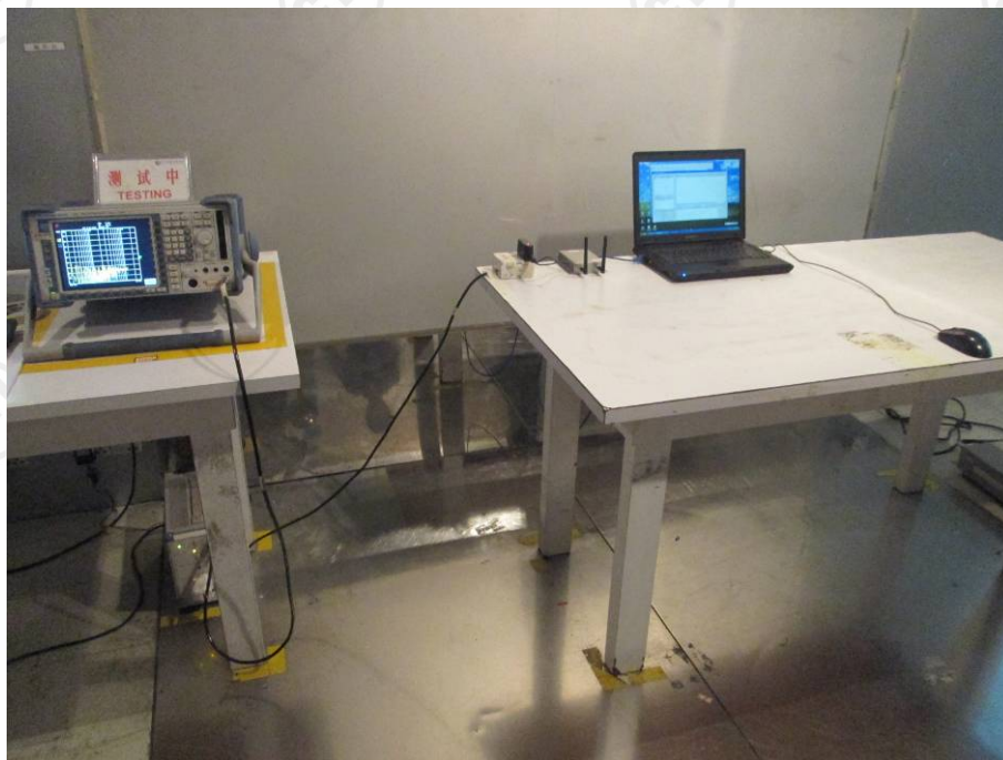
CONDUCTED EMISSION TEST SETUP
