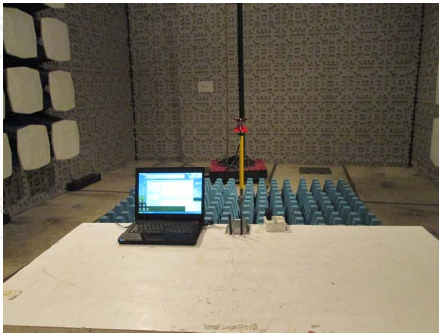
RADIATED EMISSION TEST SETUP(1GHZ-2GHZ)
