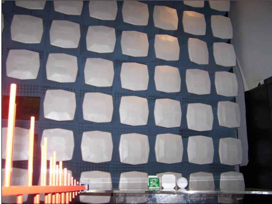
Photograph 1. Radiated Spurious Emissions, Test Setup, Below 1 GHz
