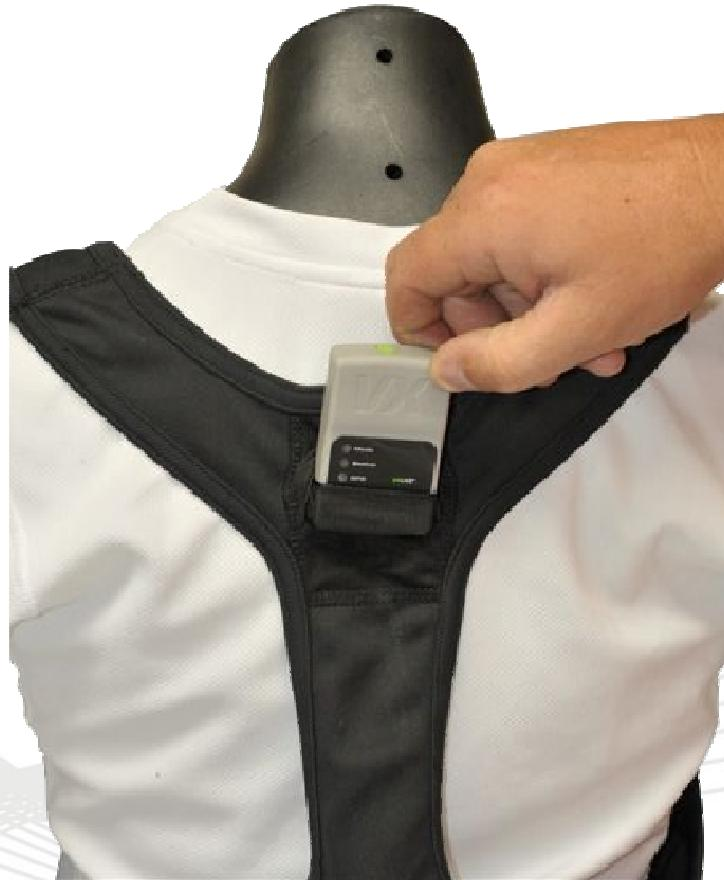
When you are finished playing or training remove the VX Log™ monitor and switch it off (by pressing the power button for at least 3 seconds).
