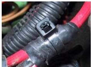
**Secure.** Place [insulation tape](#) around exposed wires. Use optional [tie wrap](#) for added security.
