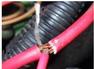
**Poke.** Use [butane soldering iron](#) or [wire cutting tool](#) to expose wires. "Poke" wires from wiring harness through vehicle wiring. See *Wiring Key*.
