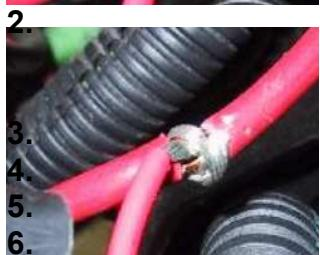
**Wrap.** Wrap wires neatly around vehicles wires.
