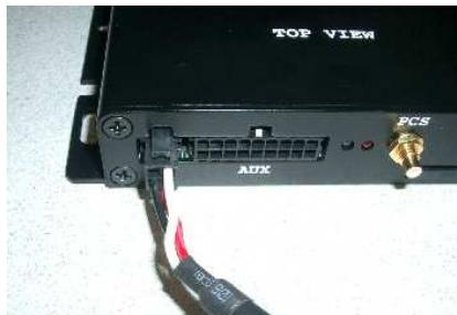
Connect wiring harness to device. Place device into an acceptable location and secure using [self-tapping screws](#) and 2 or more [tie wraps](#). It is preferable to secure device in a hidden, secure location away from moving parts.
