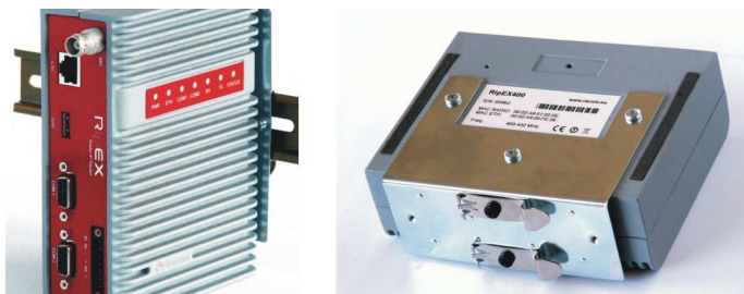
Fig. 6.3: Vertical widthwise mounting to DIN rail
