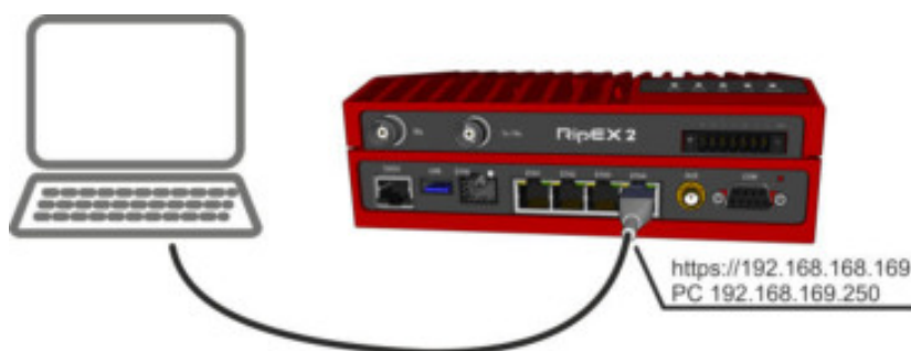
Fig. 3.6: Connecting to a PC over ETH
