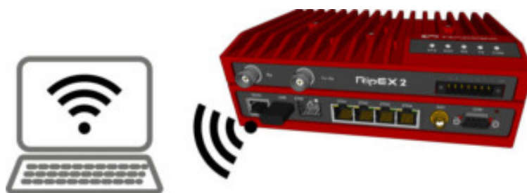
Fig. 3.4: Connecting to a PC over WiFi
