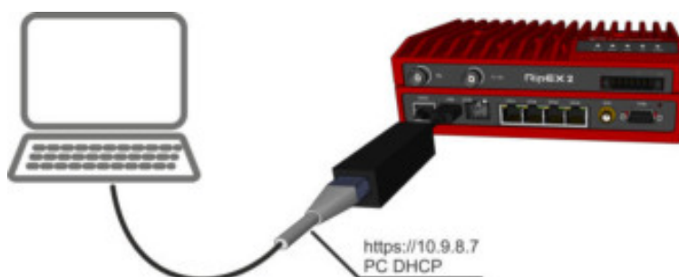
Fig. 3.5: Connecting to a PC over ETH/USB adapter
