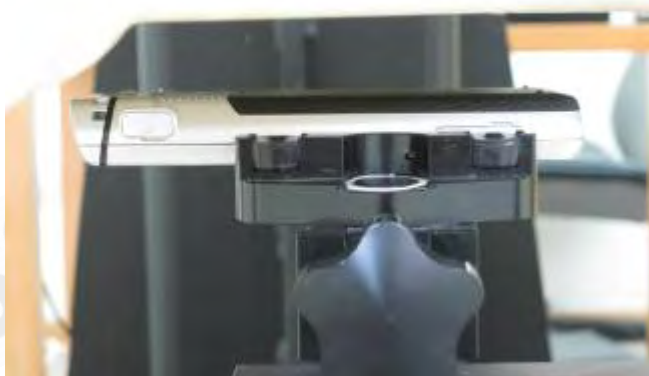
Fig.8 Body worn- EUT back to flat phantom and distance between flat phantom and mobile phone is 1.5 cm
