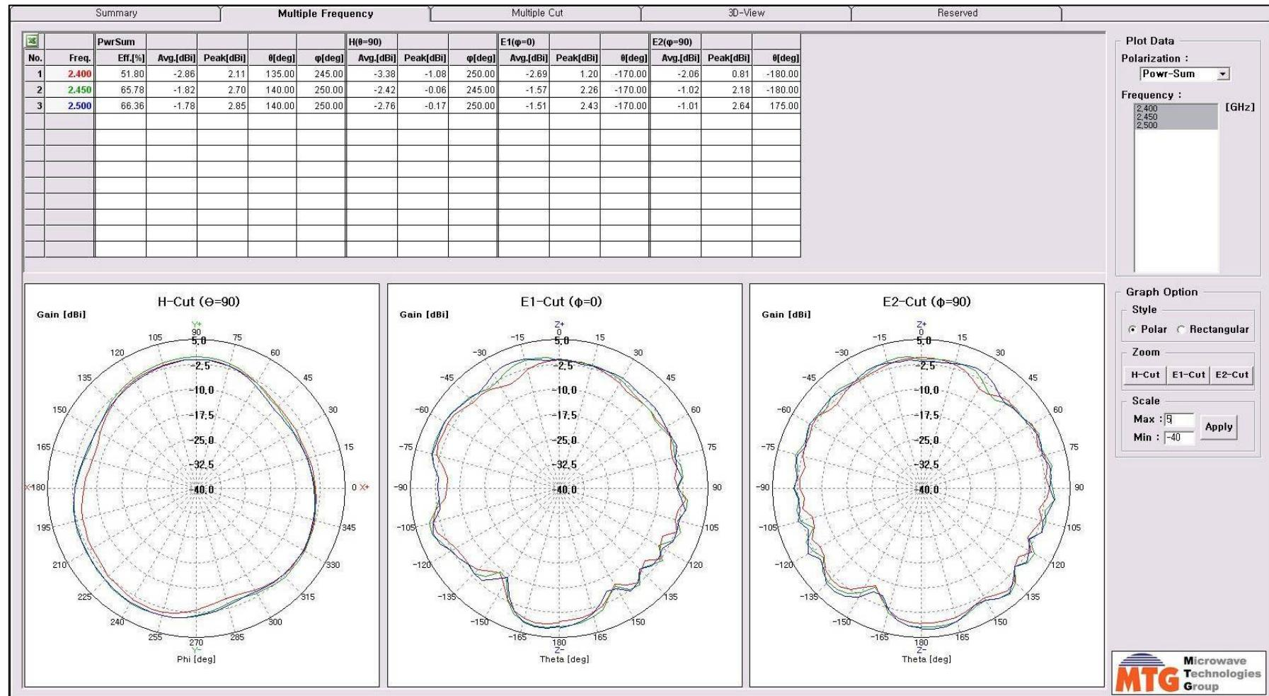
KH-WFDI-UD001 (SQ-3000 Ant) 5GHz Gain and Radiation Pattern
