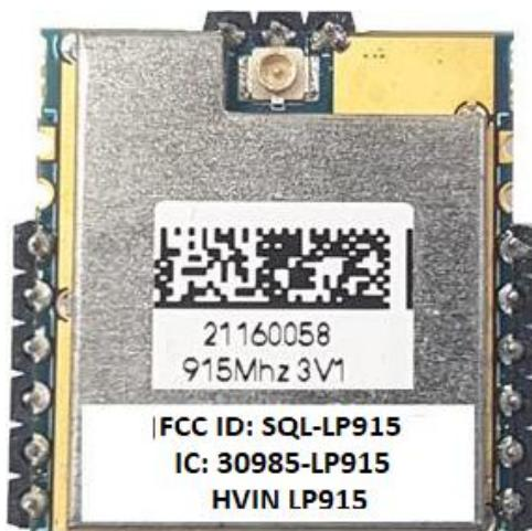
It is the responsibility of the LP915 module supplier to ensure that the LP915 module will be labelled as indicated in above image example.
