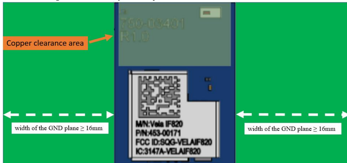
Figure 15: Integrated antenna variant layout suggestion example
