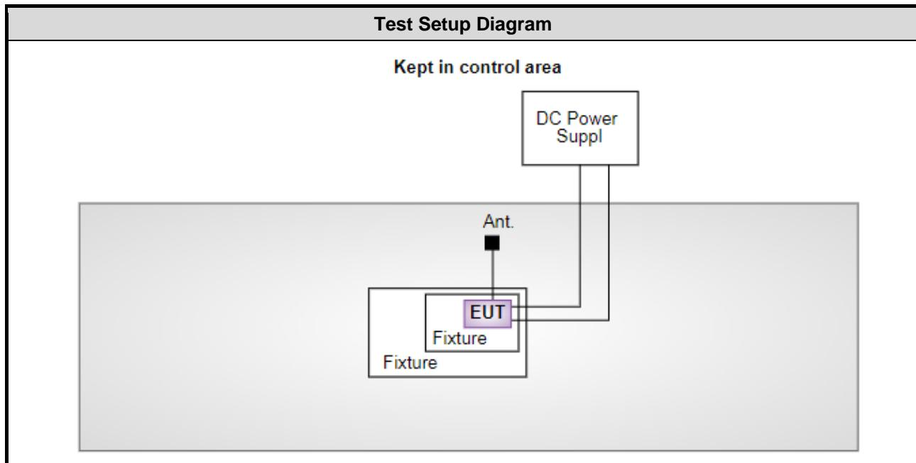
Note: The notebook and USB - RS232-G are disconnected from EUT and removed from test table when EUT is set to transmit continuously.
