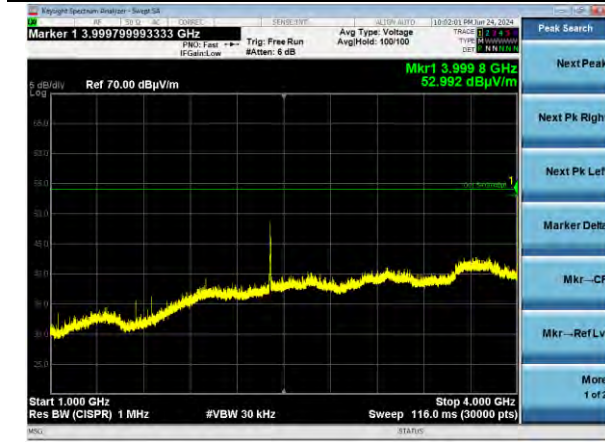
802.11a | Channel 157 | 6 Mbps | X Plane 1000-4000 MHz | Vertical
