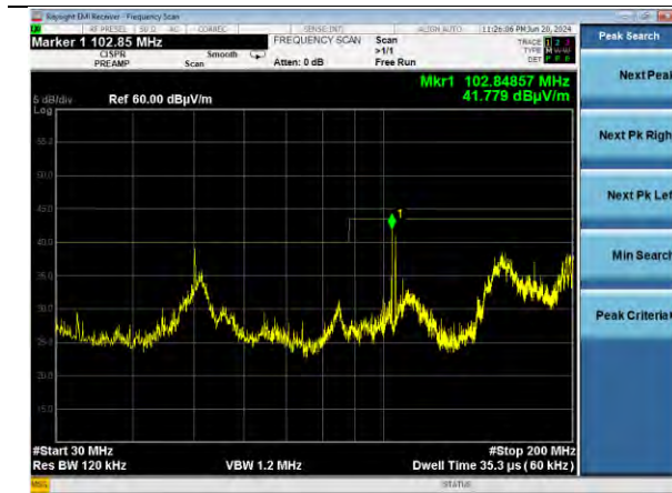
802.11a | Channel 116 | 6 Mbps | Y Plane 30-200 MHz | Vertical
