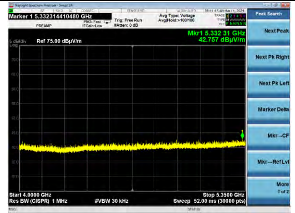
802.11a | Channel 100 | 6 Mbps | Z Plane 4000-5350 MHz | Horizontal
