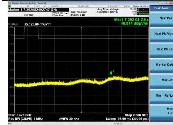
802.11a | Channel 100 | 6 Mbps | X Plane 5470-8000 MHz | Vertical
