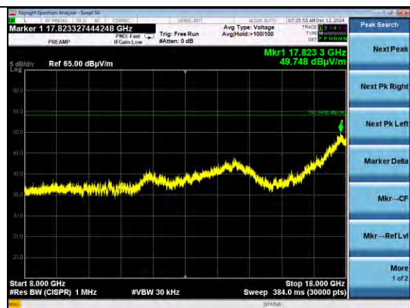
802.11ax40 | Channel 38 | MCS0 RU52 | X Plane 8000-18000 MHz | Horizontal
