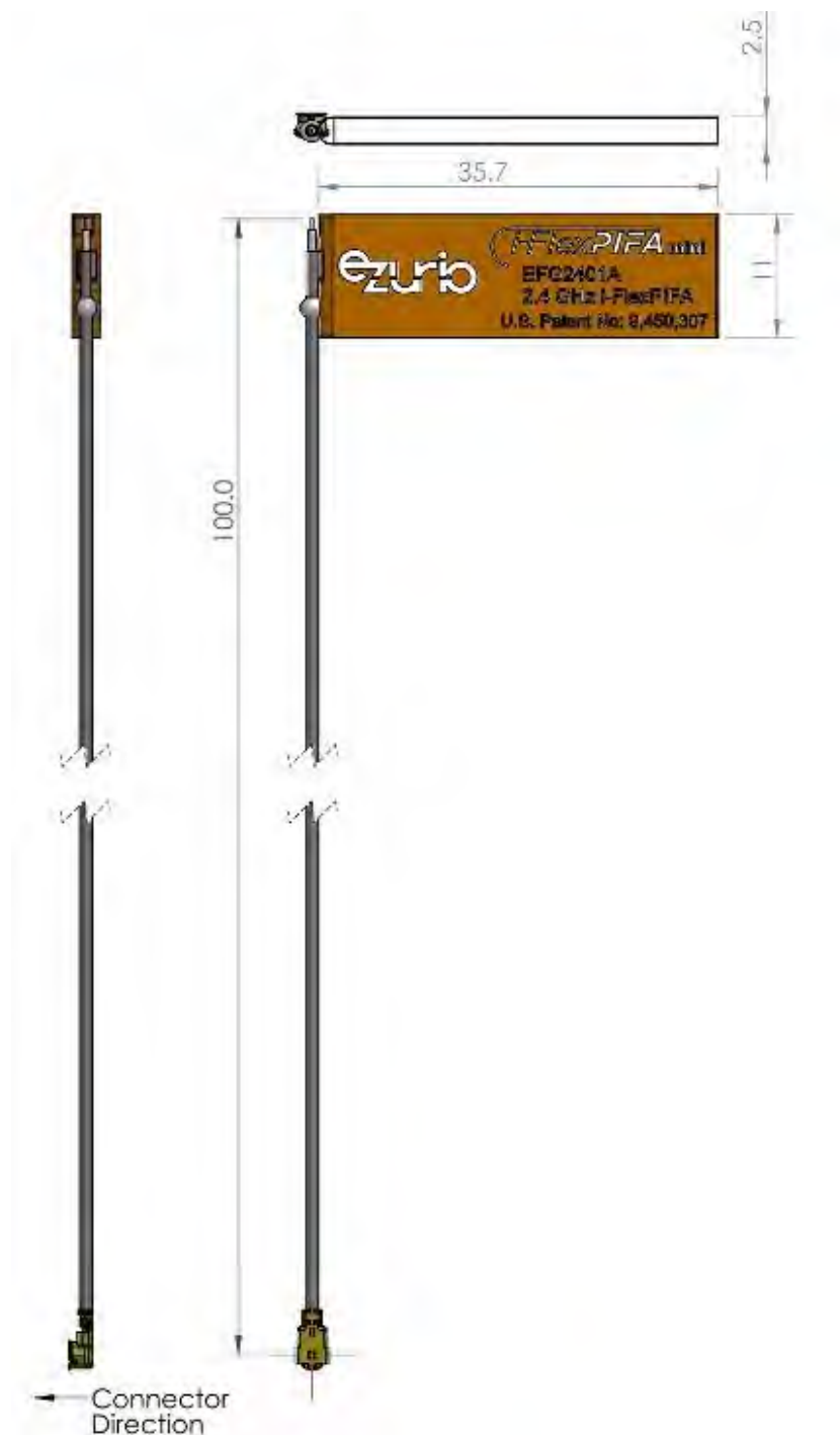
Figure 1: i-FlexPIFA mini mechanical drawing of EFG2401A Antenna
