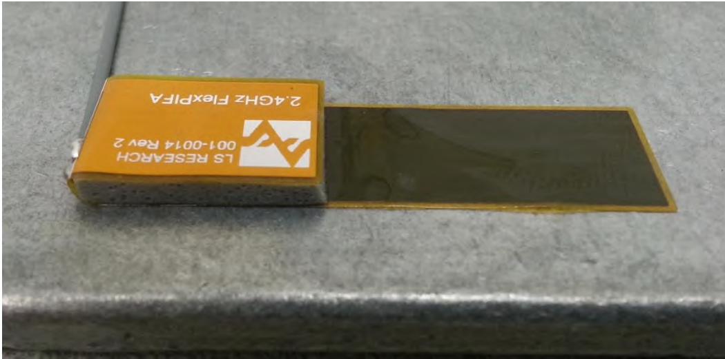
Figure 25: FlexPIFA mounted on metal
