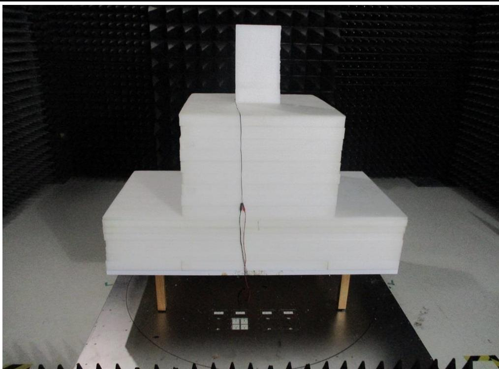
**Radiated Emission Above 1GHz Test**
