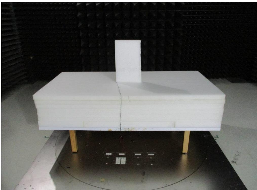
**Radiated Emission Below 1GHz Test**
