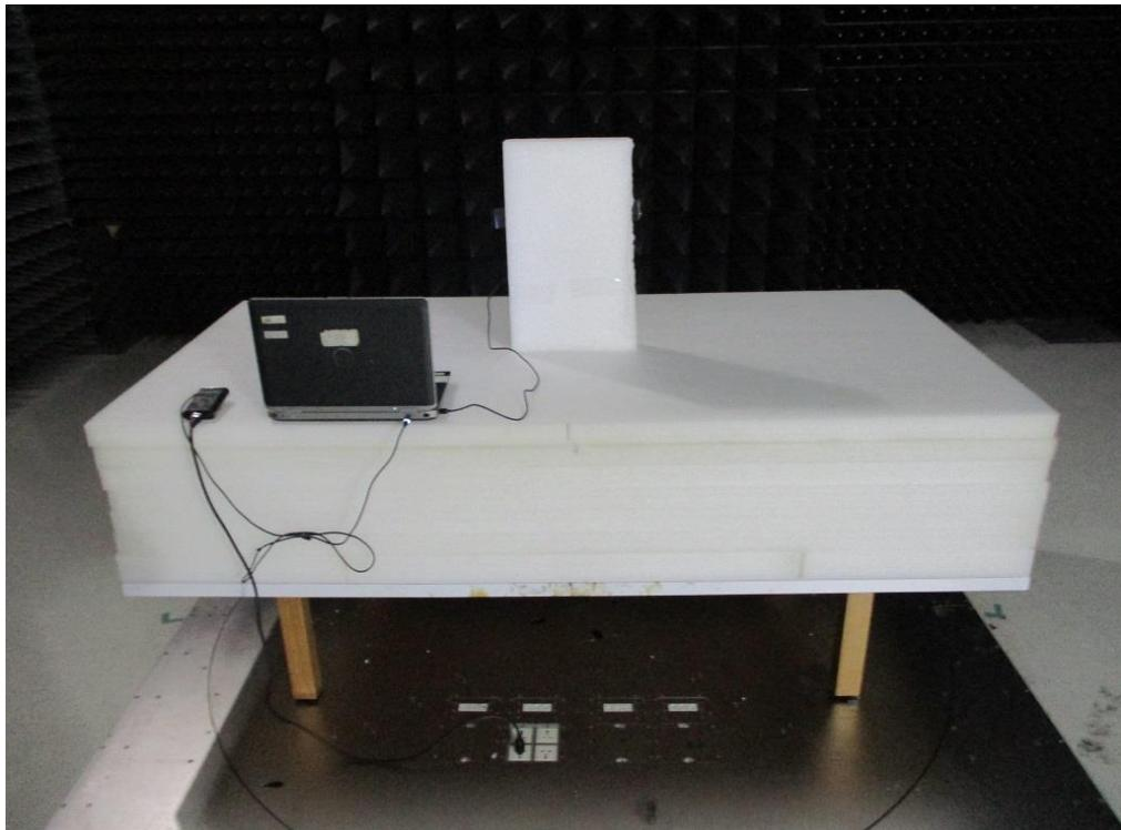
**Radiated Emission Below 1GHz Test**
