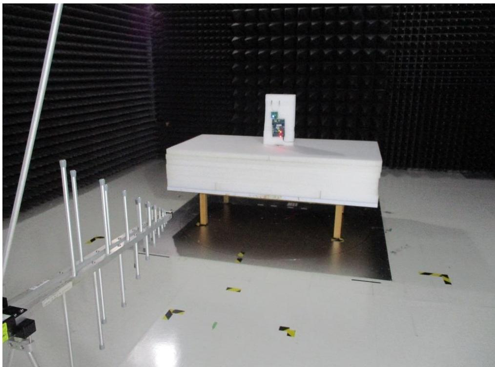
**Radiated Emission Above 1GHz Test**
