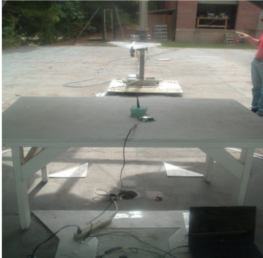
Photo 4. Test Setup 200 MHz to 1000 MHz testing.
