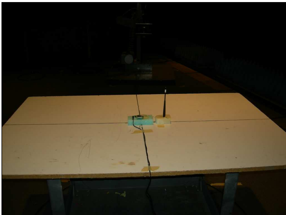
Figure 2: Radiated Emissions Test Setup – XPOS
