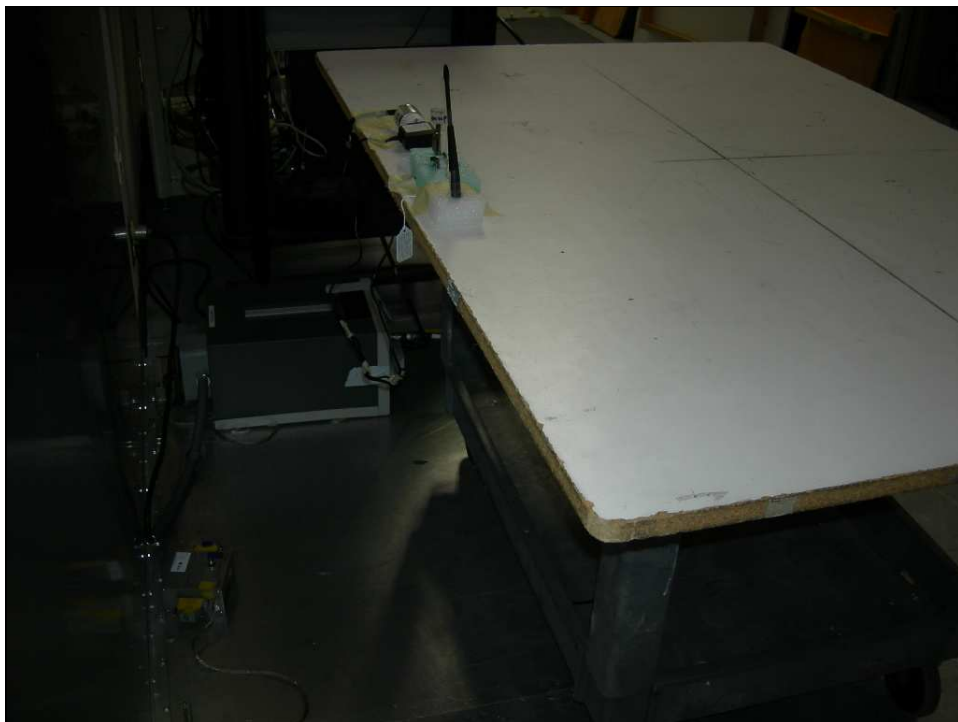
Figure 8: Conducted Emissions Test Setup – ZPOS
