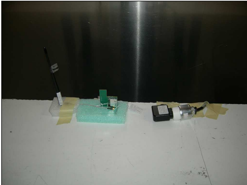
Figure 7: Conducted Emissions Test Setup – ZPOS
