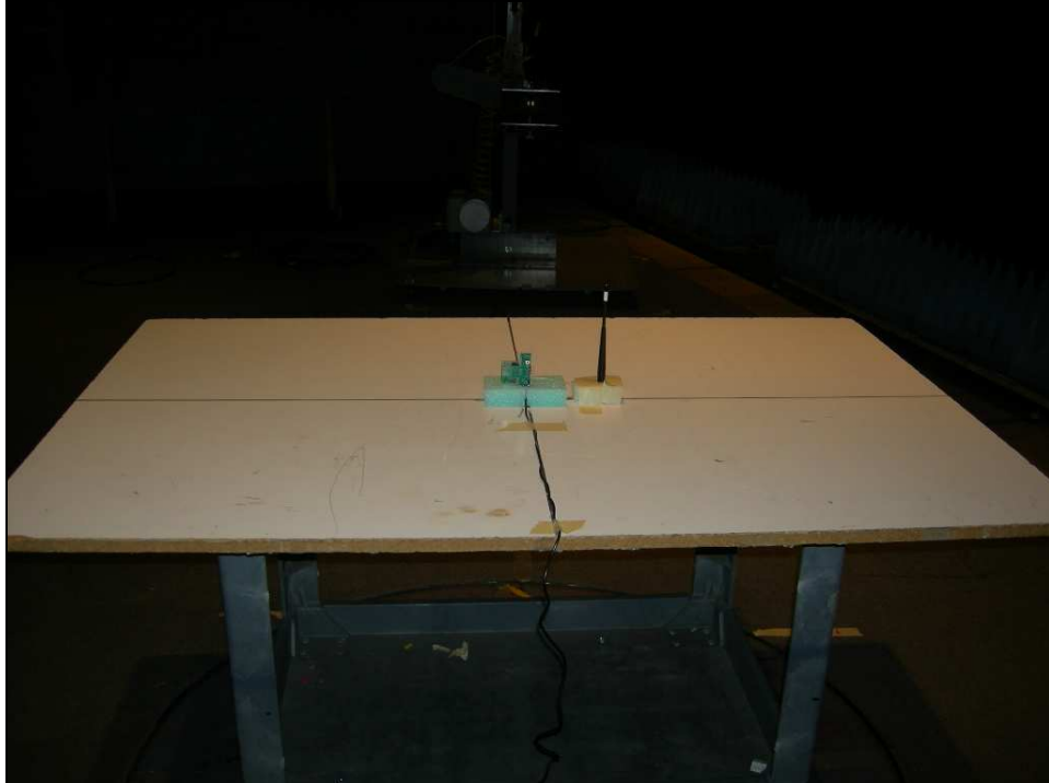
Figure 6: Radiated Emissions Test Setup – ZPOS
