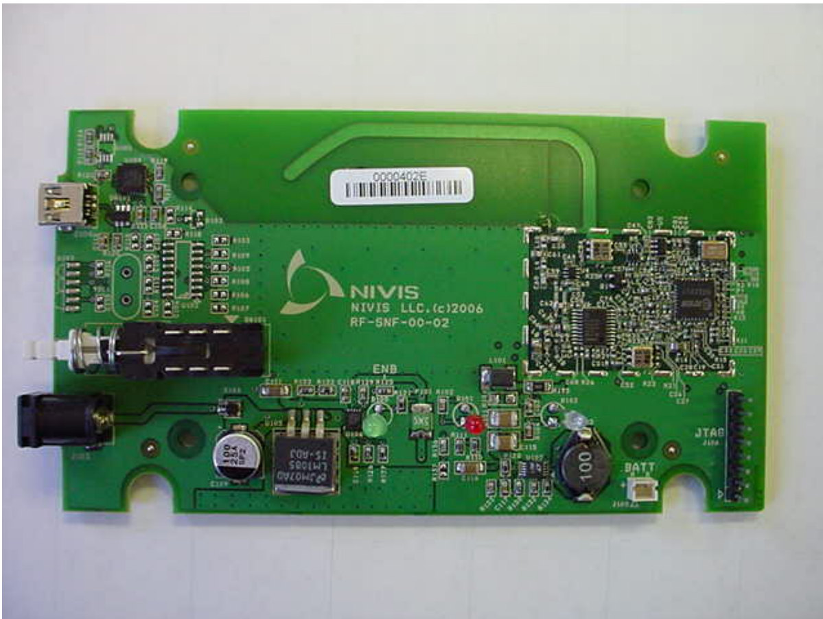
Photo Two – Internal RF Section
