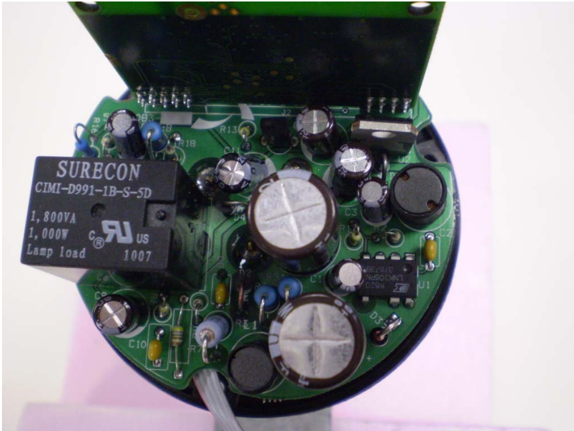
Photo Three – Internal Top View of Board on which the Radio Board Sits
