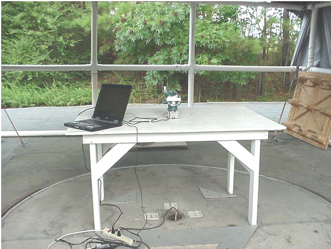
Figure 3: Radiated Test Configuration Antenna 2 Antenna 2.0dBi Gain (Front View)
