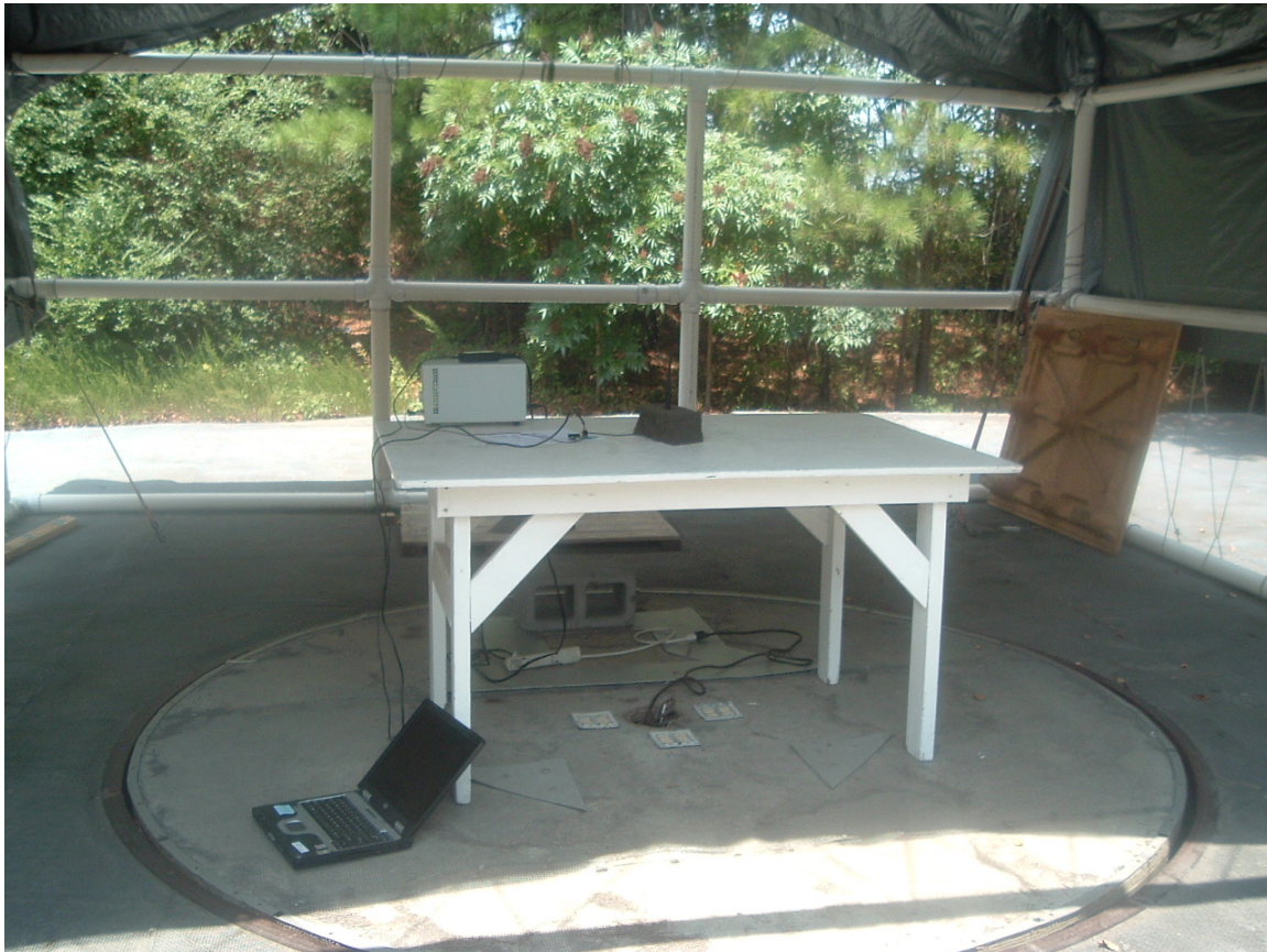
Figure 1: Radiated Test Configuration Antenna 1 Omni Antenna 5.0dBi Gain (Front View)
