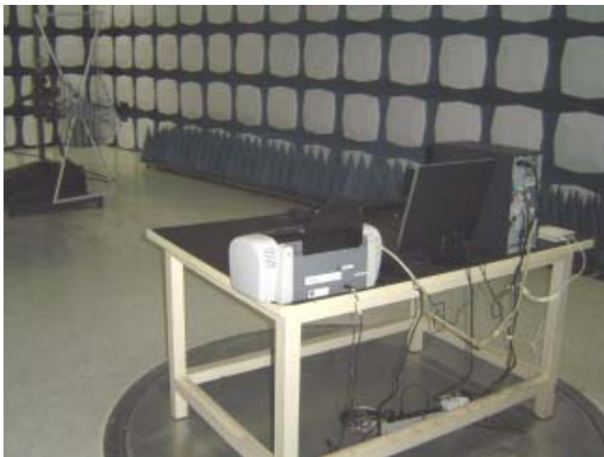
Radiation Emission Test Setup View for 15" Monitor Back
