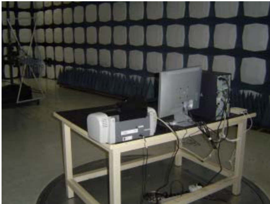
Radiation Emission Test Setup View for 17" Monitor Back
