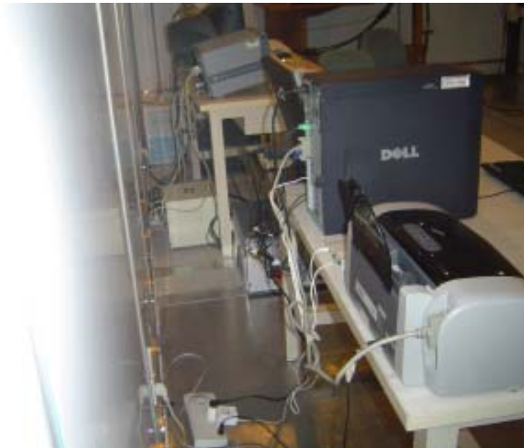
Conducted Emission Test Setup View for 15" Monitor Back
