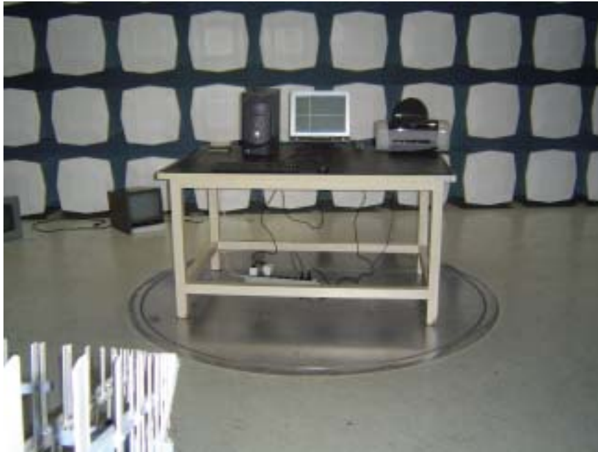
Radiation Emission Test Setup View for 15" Monitor Front
