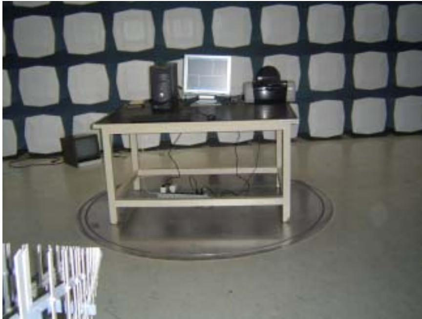
Radiation Emission Test Setup View for 17" Monitor Front
