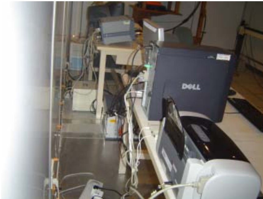
Conducted Emission Test Setup View for 17" Monitor Back
