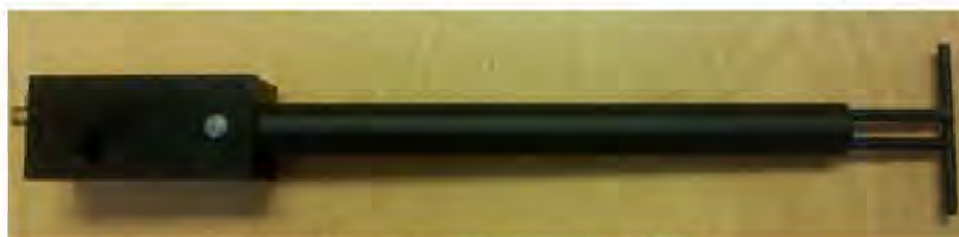
Figure 1 – MVG COMOSAR Validation Dipole
