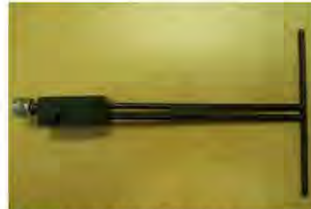
Figure 1 – MVG COMOSAR Validation Dipole
