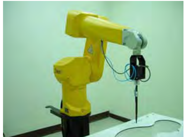
Fig. 5.2 Probe setup on robot
