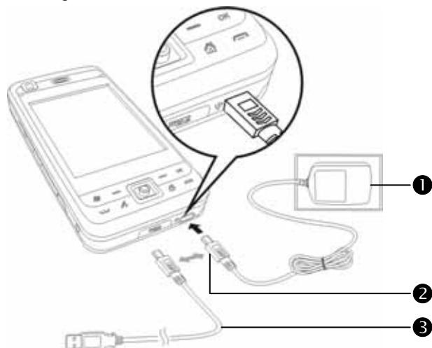
1. It will take about 8 hours to fully charge the battery after the first time you open the package. Subsequent charging will only take about 3 hours. After charging, you can disconnect the AC adapter and carry the Pocket PC around portably. To maintain smooth operation, charge the power regularly.
