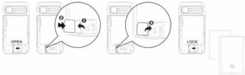
4. **Installing the Battery**
