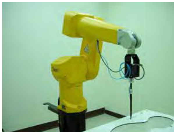
Fig. 5.2 Probe setup on robot
