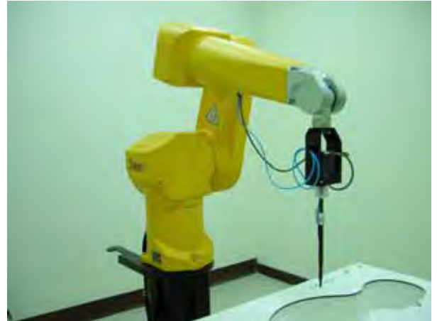
Fig. 5.2 Probe setup on robot
